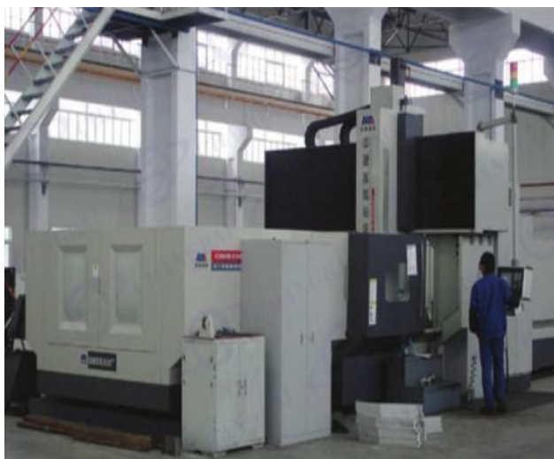
CNC Gantry Boring & Milling Machine TK422 2000x4000
